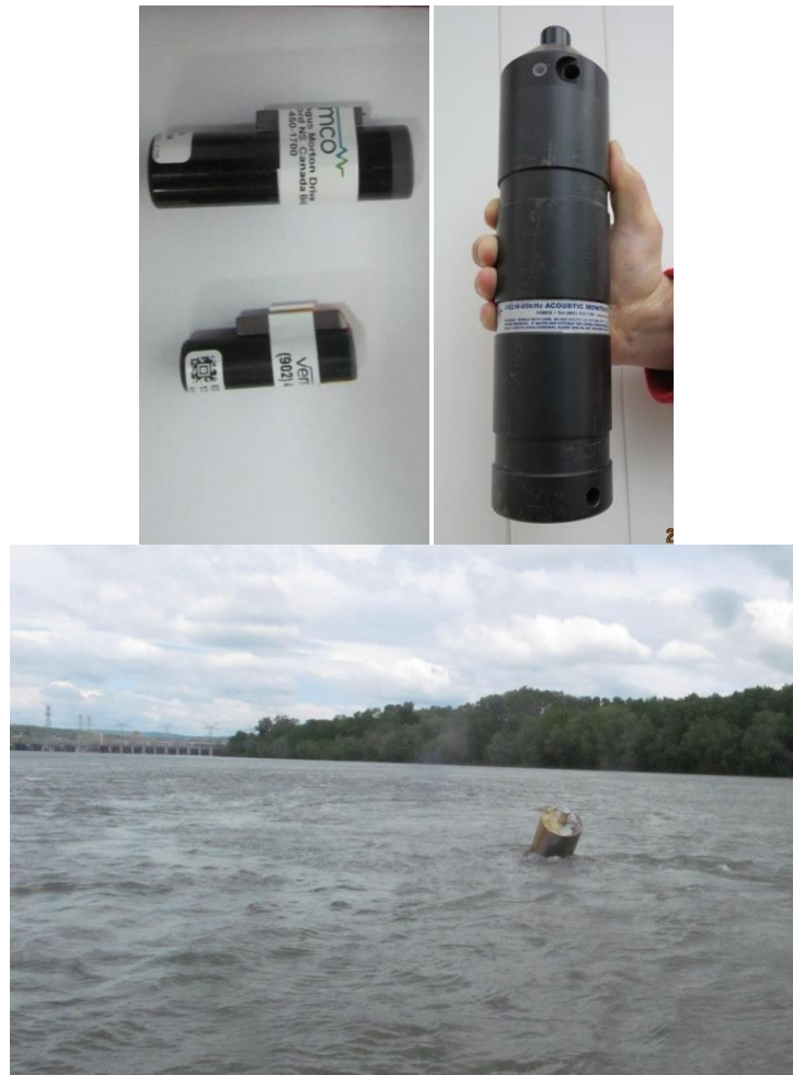
Figure 2: Equipment used for fish tagging (9 mm & 13 mm Vemco tags) - left; VR2W receiver - middle; buoy used to install receivers in the river downstream the dam – right
